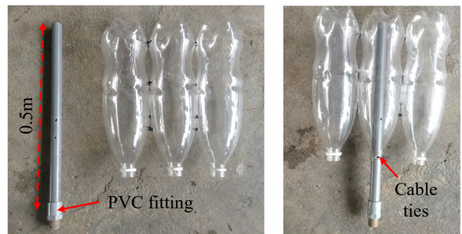
Fig. 1. Blade parts of BOWW.
