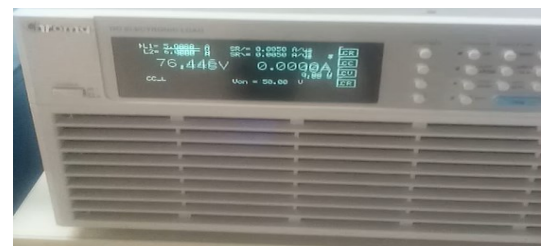
Fig. 7. Results of maximum output voltage measurement without a load.
