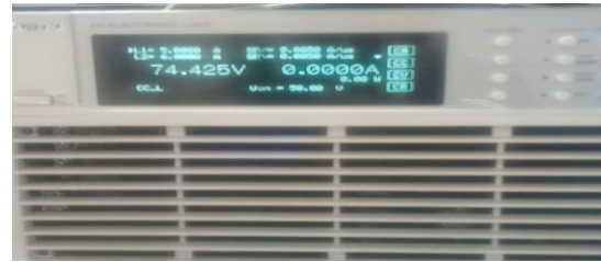
Fig. 6. Results of minimum output voltage measurement without a load.
