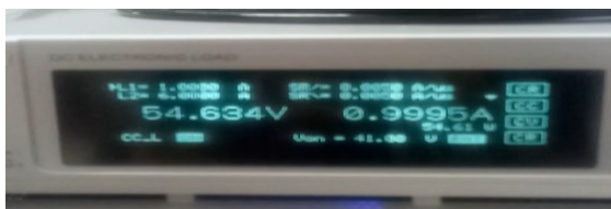
Fig. 9. Experimental results for 1 A load current.
