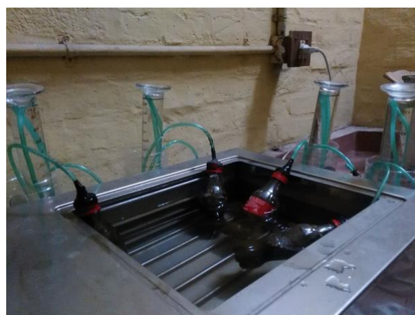
Figure 1. Gas production reactor (coca cola bottle) in water bath
