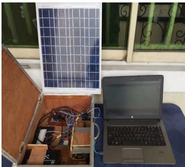
Fig. 4. Experimental setup for data collection using SIMMM-PVS without soot In Akwa, Anambra state.
