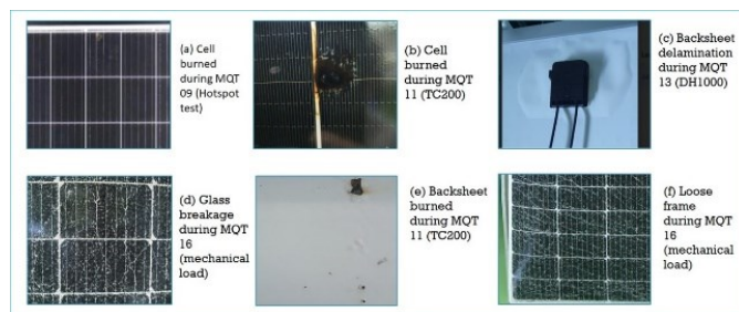
Fig. 6. Visual failure from the test results.
